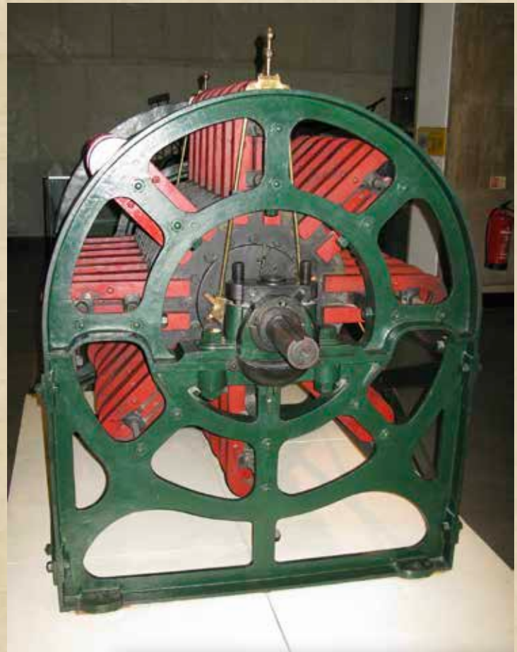
ABOVE: The electrical generator designed by Holmes and installed at Souter Point. The first of many designs that appeared in quick succession once the principles had been established, this was very similar to the one trialled at South Foreland.
